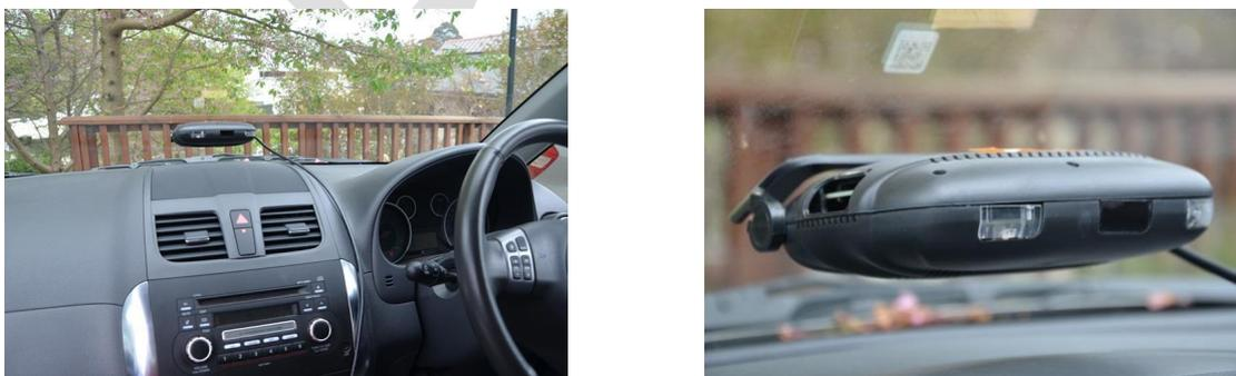
*Figure 8: Image of cabin interior of pilot study vehicle showing window mounting (left) and close-up (right) of miniDAS device*
